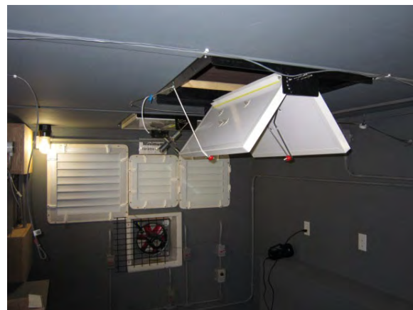
Figure 2. Trailer end-wall exhaust fans (left) and interior room showing ceiling inlets (right).
