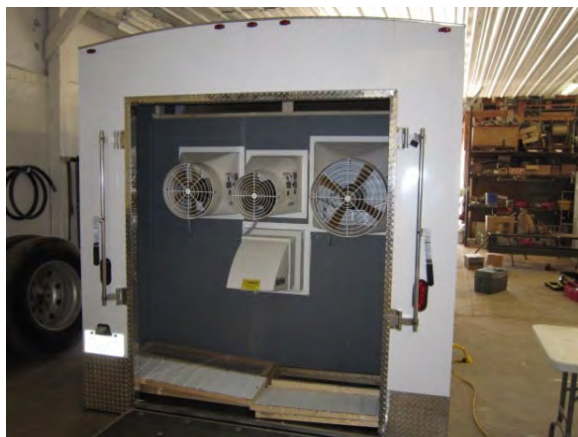
Figure 2. Trailer end-wall exhaust fans (left) and interior room showing ceiling inlets (right).
